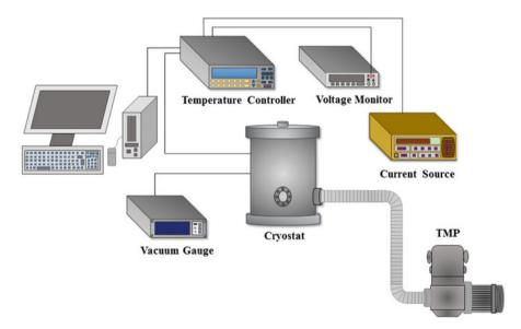
Fig. 11.2 Scheme of the electrical measurement setup
