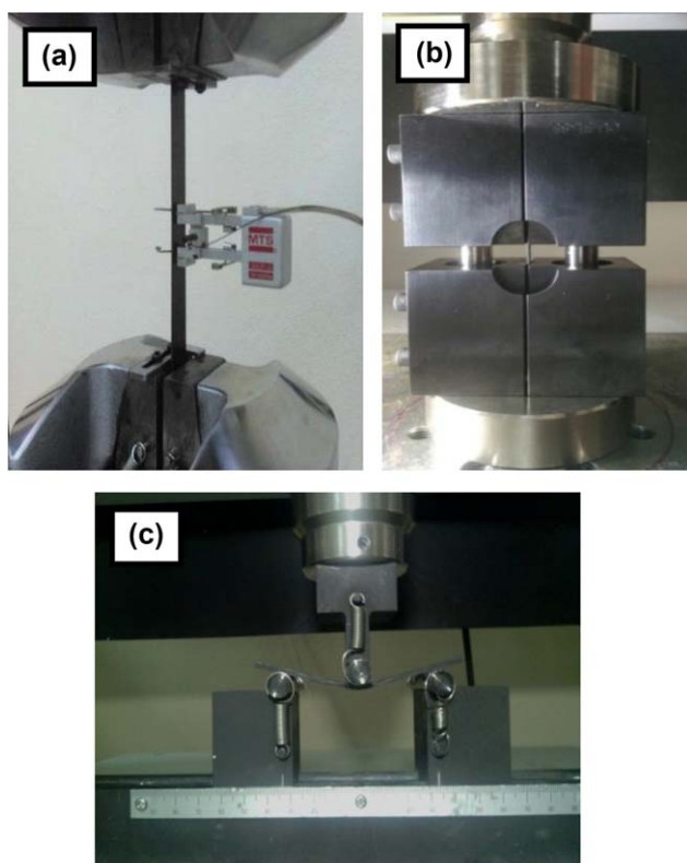
Figure 5. Photographs of the test specimens under (a) tensile and (b) compressive loading and (c) three-point bending. [Color figure can be viewed at wileyonlinelibrary.com]
