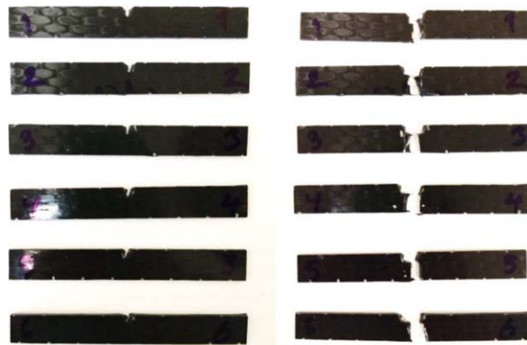
Figure 8. Composite test specimens before and after impact loading. [Color figure can be viewed at wileyonlinelibrary.com ]
