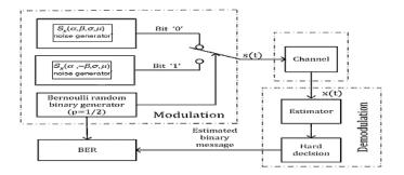
Fig. 1. Block diagram of the random communication system.
