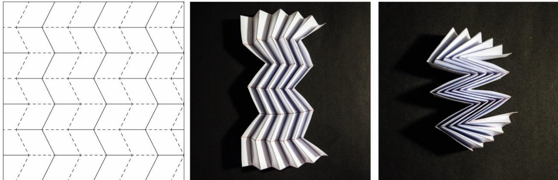
Figure 2.23. Miura-ori pattern / Herringbone pattern – drawn based on (Source: Miura, 2009) and folded by the author.
