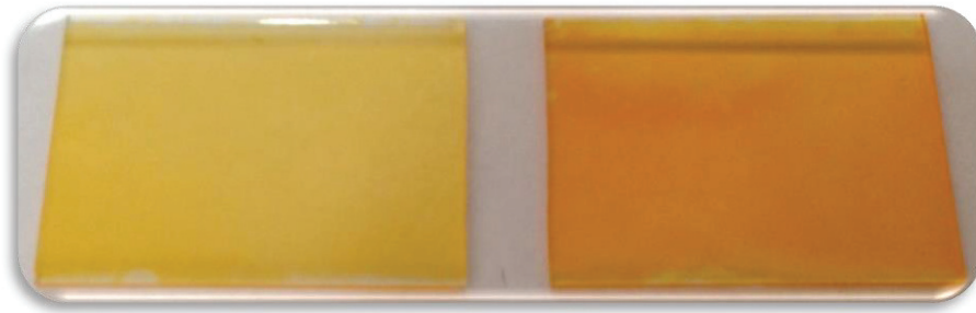
Figure 5.8. CdS coated glass substrates; the yellow one (on left) is thin and the orange one (on right) is thick film.
