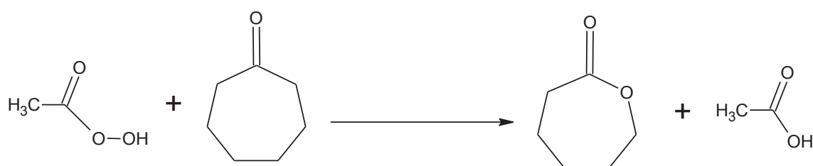
Figure 2.4. The commercial production of \epsilon -caprolactone monomer from Baeyer Villiger oxidation method (Source: Labet and Thielemans, 2009).
