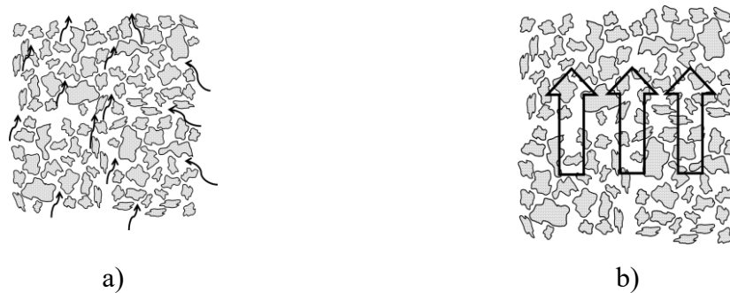
Figure 1.3. Two main approaches employed for heat and fluid flow simulations in porous media; a) Pore Scale Method (PSM), b) Volume-Averaged Method (VAM)
