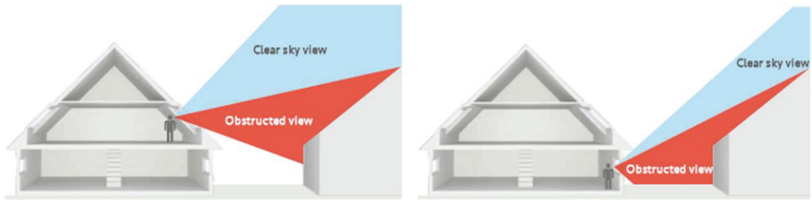
Figure 2.2. Components of view-roof window and view-facade window situation. (Source: Ruck et al., 2000)
