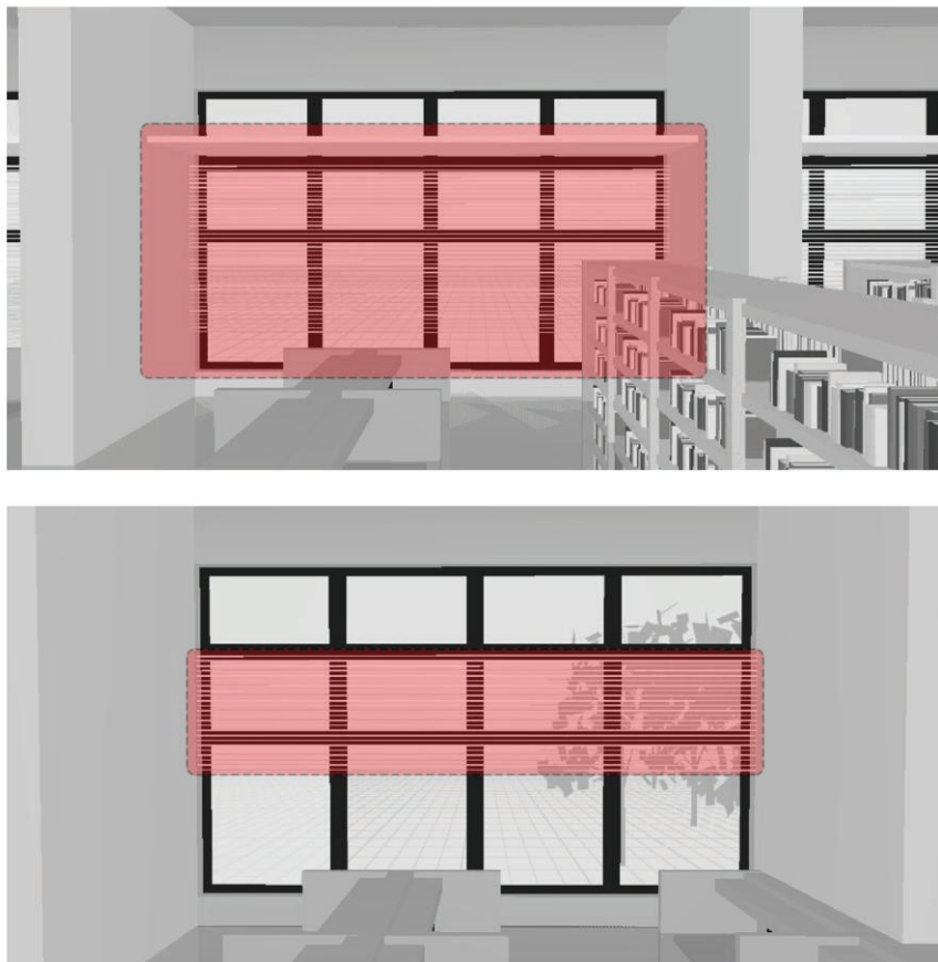
Figure 3.8. The application of the light shelf-reflective louver system on south-west facing window (above) and the reflective louver system on north-east facing window (below).
