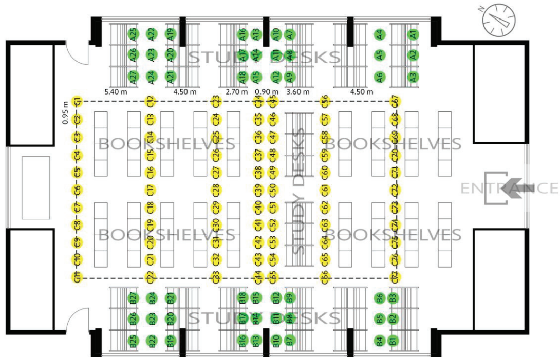
Figure 3.3. The determined on-site monitoring points for the horizontal illuminance measurement.
