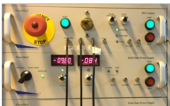
Figure 5.7. Control panel of PEF equipment
