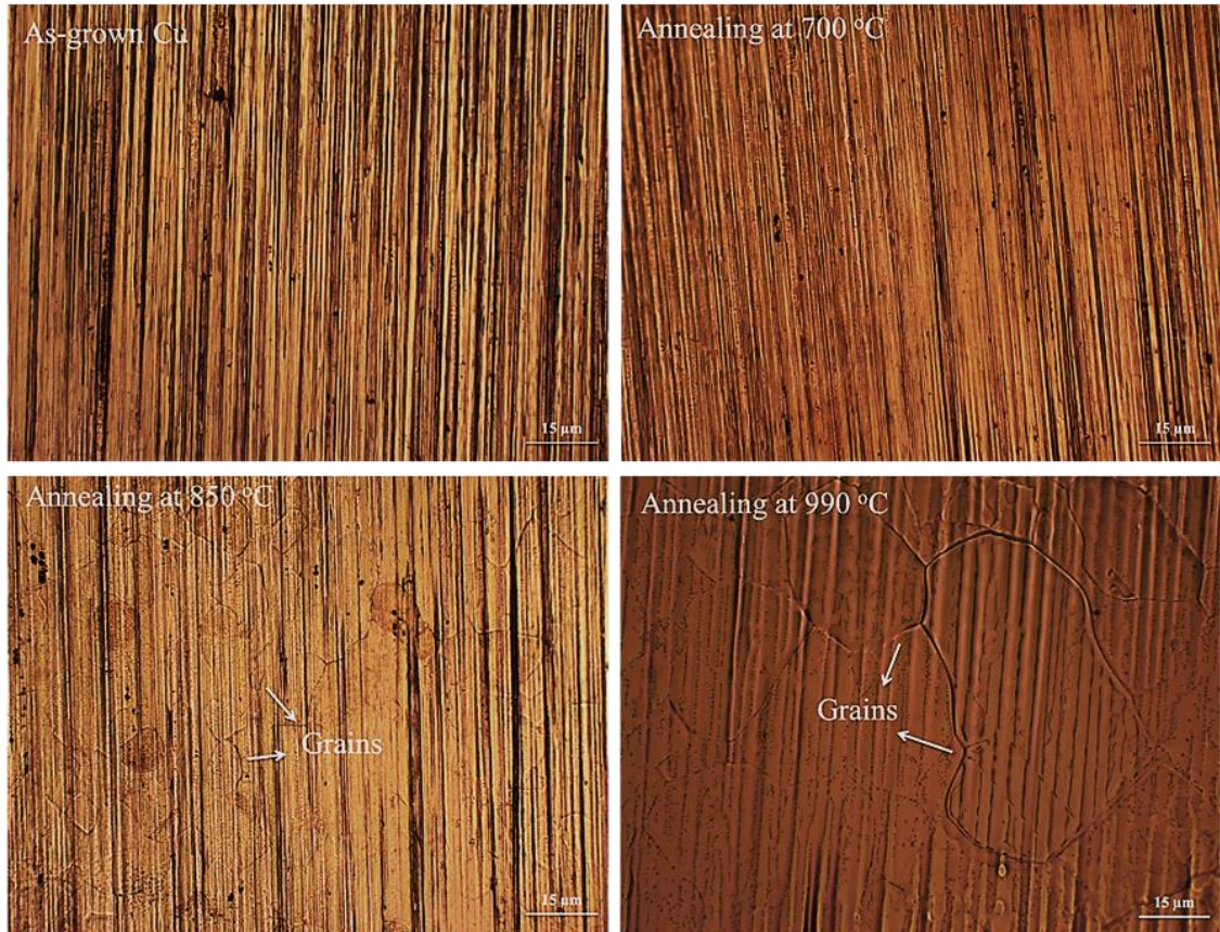
Figure 25. Change in grain size and formation based on different annealing temperatures; (a) 700 °C, (b) 850 °C and (c) 990 °C viewed by using 10x optical microscope.
