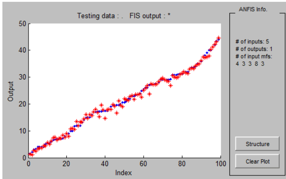
Figure 5.11. The comparison of ANFIS study with software model output (in red stars) and actual experimental outputs (in blue dots) after revisions of dataset
