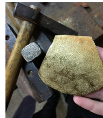
Different patterns were given by hitting with hammer.
