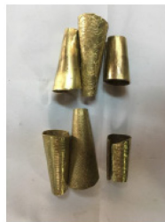
To make the six sheets conical, it was shot with a hammer.
