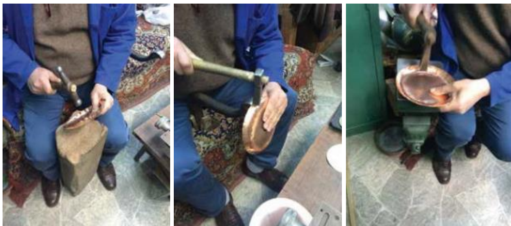
Figure 4.29. Hammering process :Turning a flat metal into a 3 dimensional shape (Photography: İrem Altunsu) (cont. on next page)
