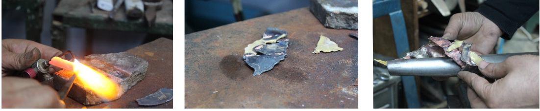
Figure 4.38. Welding and melting all the edges to create color change.
