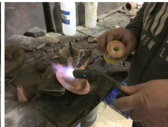
Feets were soldered to the top of the product.
