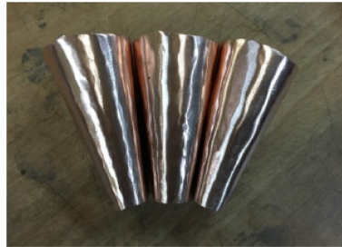
All parts of feet were smoothed and polished with sanding.
