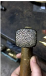
The feet were patterned with hammer.
