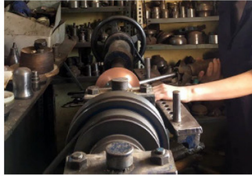
The mold was found, which is suitable for the design. And metal spinning was made with using the mold.
