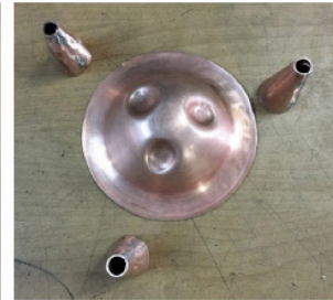
To make copper conical, it was shot with a hammer. Welding was done to combine the two ends.
