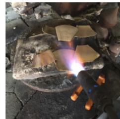
The six sheets were annealed.
