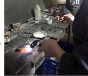
To make copper conical, it was shot with a hammer. Welding was done to combine the two ends.
