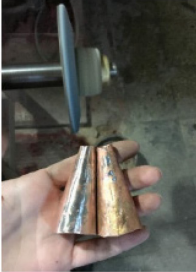
To remove the weld marks the feet were sanded.
