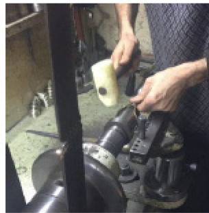
Trials for beating on different surfaces. Spinning and beating.
