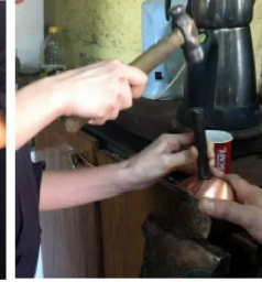
Three points of the product were hollowed out with a hammer.
