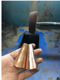
To remove the weld marks the feet were sanded.
