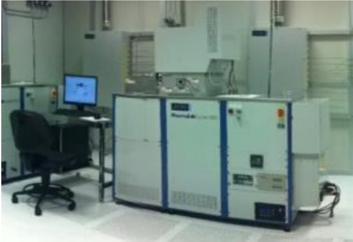
Figure 27. Oxford PlasmaLab 100 ICP 300 ICP-RIE System in Sabancı University Nanotechnology Research and Application Center (SUNUM) used for dry anisotropic etching of 6H-SiC based samples retaining Cr/Ni nanoisland hard mask on their surfaces.
