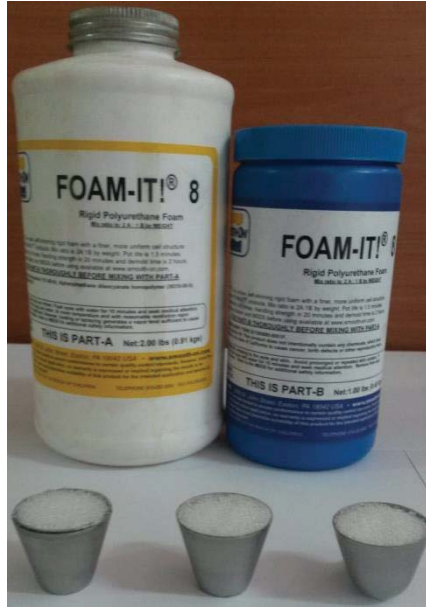
Figure 3.8. Two-component rigid polyurethane foam and foam-filled core geometries.
