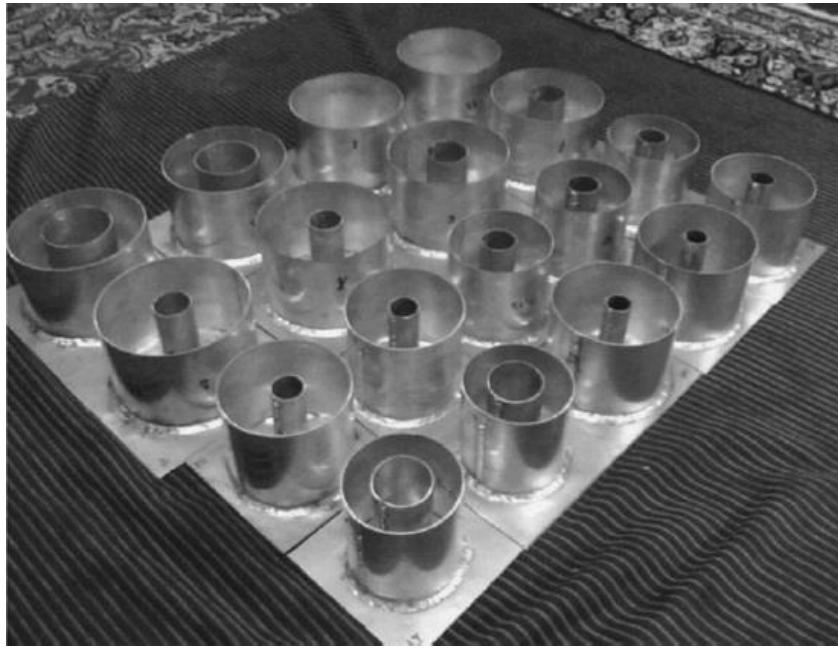
Figure 2.20. Tested bi-tubular concentric thin-walled cylinders with different radial distances (Alavi Nia & Khodabakhsh, 2015)
