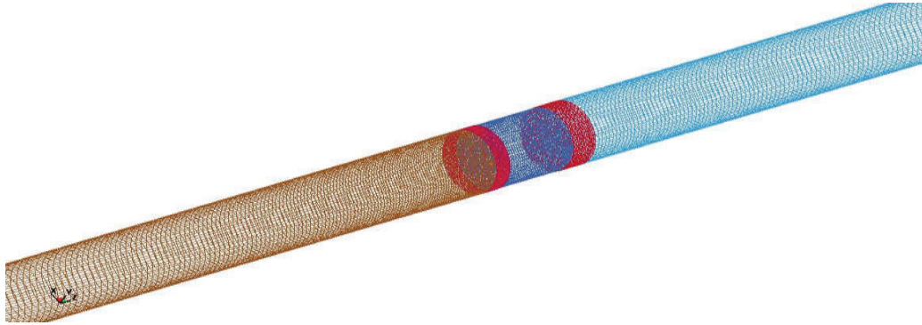
Figure 2.24. Numerical model of SHPB test setup
