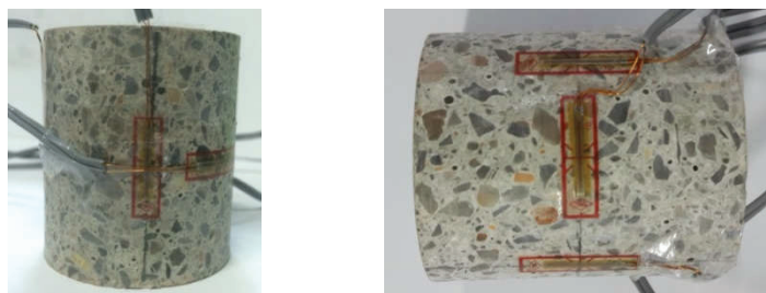
Figure 2.9. Strain gauges glued on the axial and circumferential directions of the specimen
