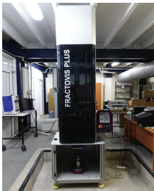
Figure 3.3. Drop tower testing device
