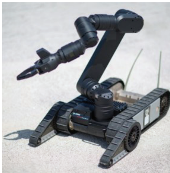
Figure 2.2. RedHawk MPR mobile robotic system with haptic control (Source: Harris Robotic Systems, 2016).
