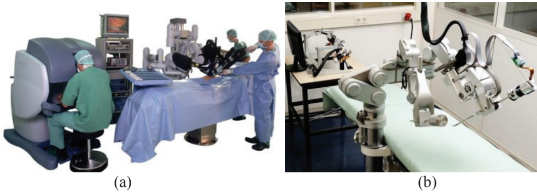
Figure 2.1. (a) da Vinci surgical robot (Source: Intuitive Surgical, 2016), (b) Sofie surgical robot (Source: Bedem, 2010).
