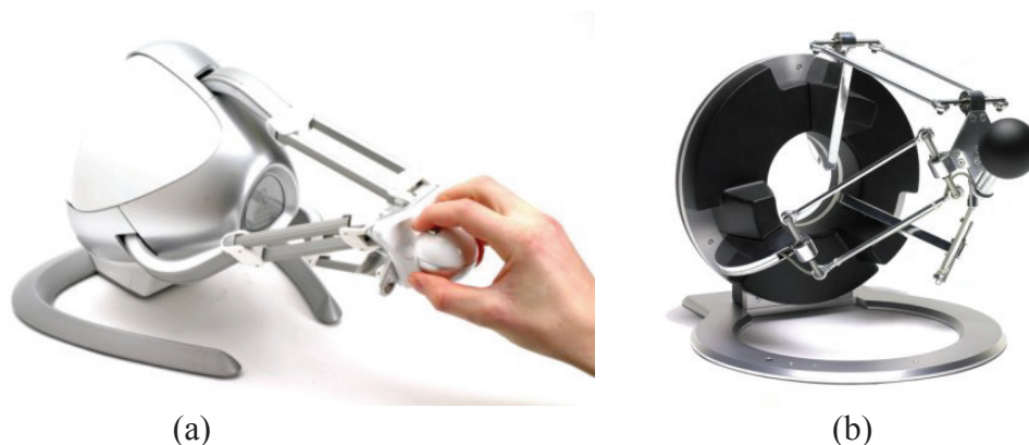
Figure 2.4. (a) Novint Falcon haptic device (Source: Novint Technologies, 2016), (b) omega.3 (Source: Force Dimension, 2016).
