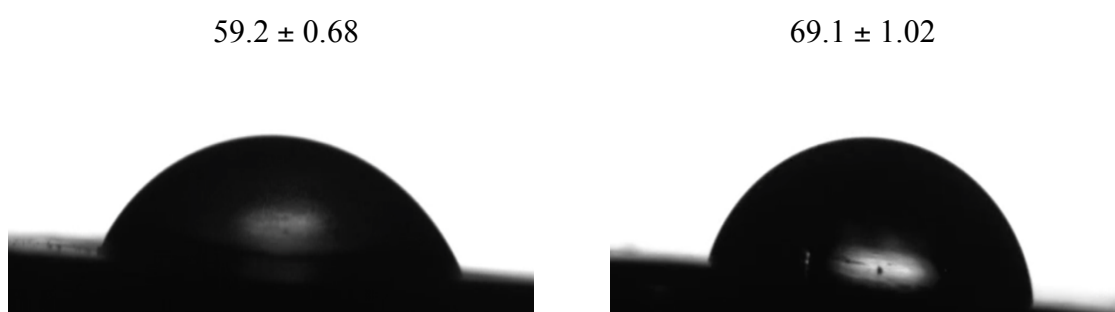
Figure 4.20. Contact angle measurement of support with PSF:SPES ratio a) 4:1 and b) 5:1.
