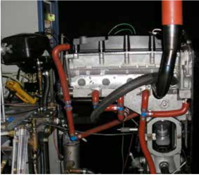
Figure 2. View of single cylinder optical engine
