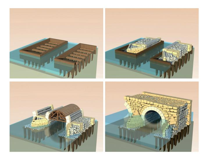
**Figure 14.** Construction of foundation system; perspective view from the 3D reconstitution model
