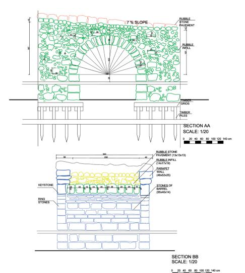
Figure 12. Reconstitution drawings of the structural system, 2D detail drawings
