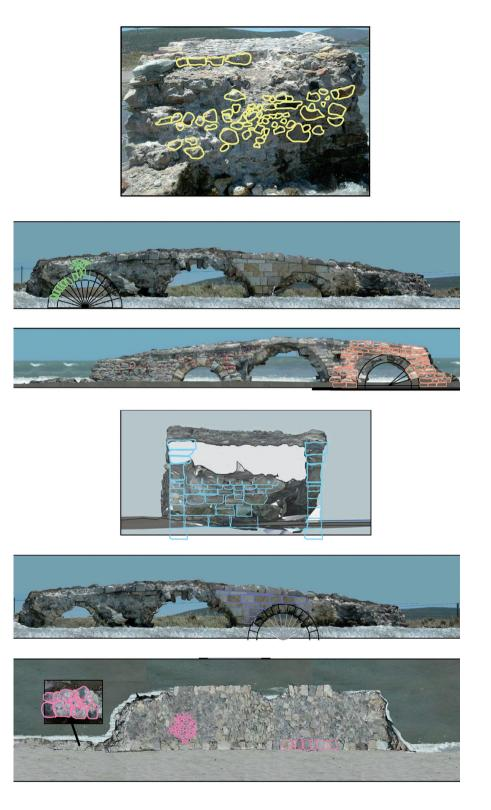
Figure 10. Sources of reconstitution, orthogonal views from the 3D survey model
