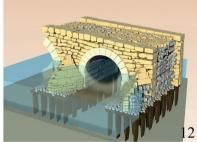
**Figure 13.** Possible sequence of the original construction; perspective views from the 3D reconstitution model
