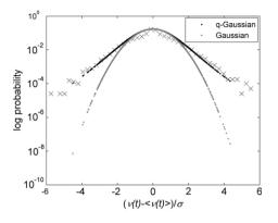
Fig. 9b. Semi-log plot of speed difference time series, fitting plots of Gaussian and q-Gaussian forms.
