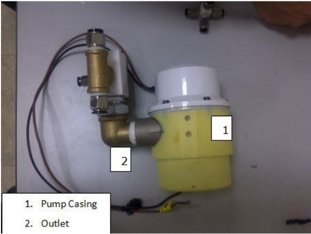
Figure 9: Pump and Distributer
