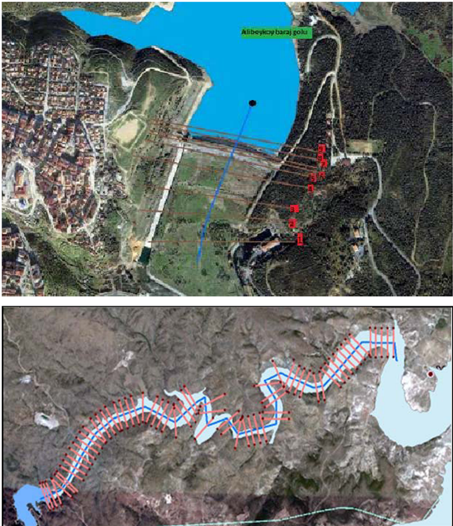
Fig. 6 Cross sections used in modeling of 1D flow of flood propagation via HEC-RAS along the Alibey and Porsuk creeks after the Dam-break
