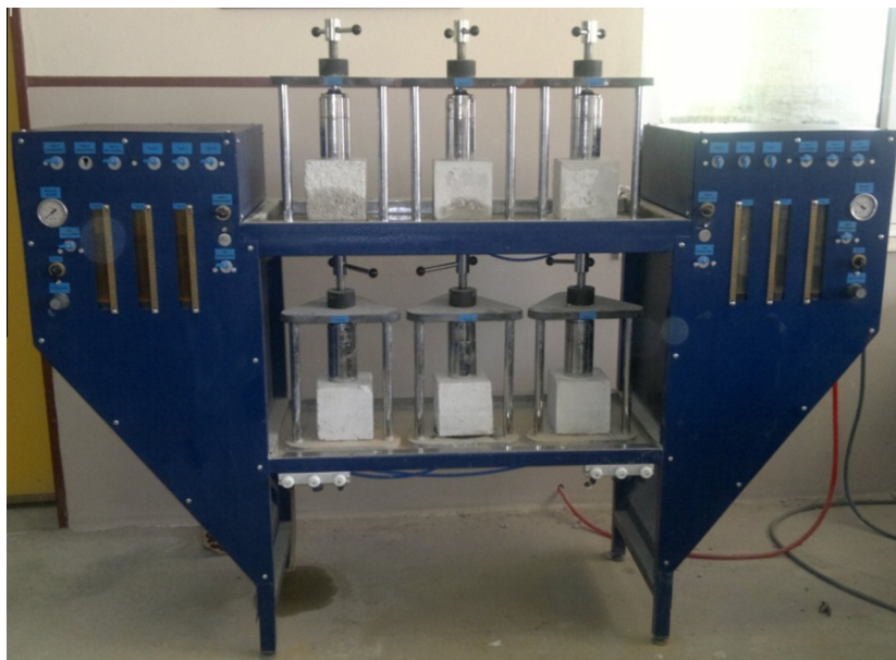
Fig. 2. Permeability test set up for determining the water penetration depth.
