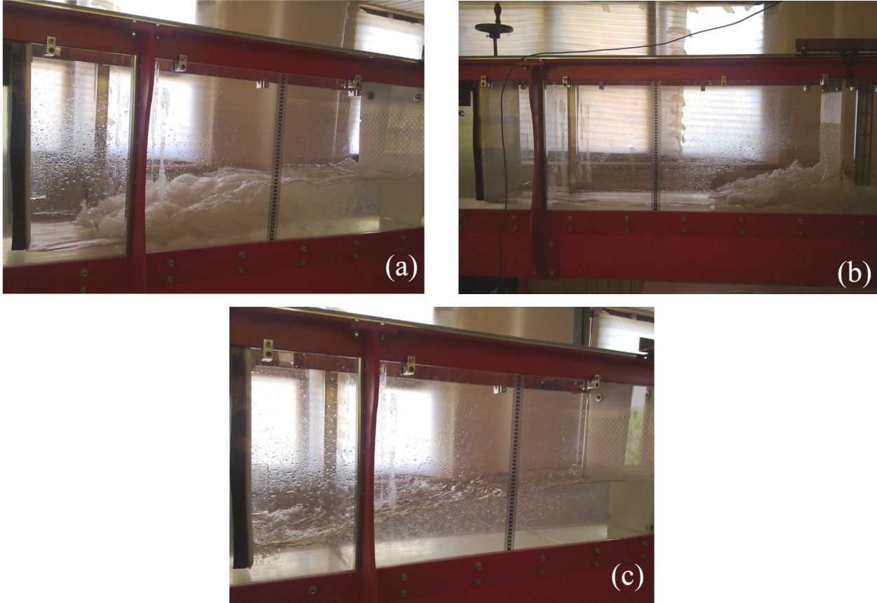
Figure 1. Different behaviors through collision of supercritical flow with screens: (a) first type, (b) second type, (c) third type.
