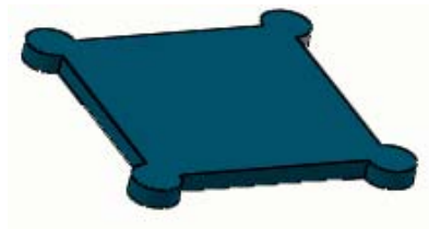
Figure 4.57. Square plate with four hinges
