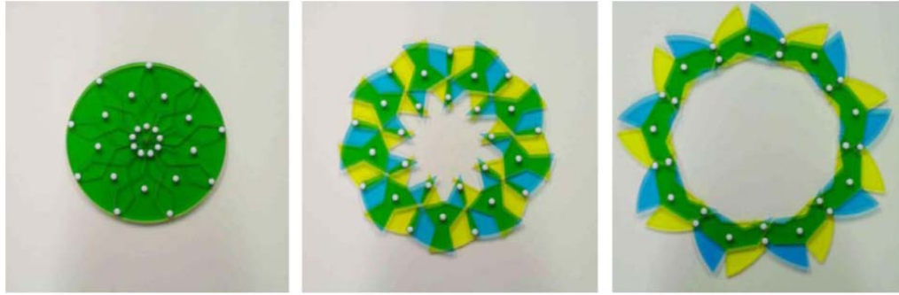
Figure 2.20. Expansion sequence of an RPS with a polygonal opening (Luo, et al. 2007)
