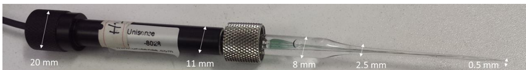
Figure 2.3. The dimensional size of the Unisense Microsensors.
