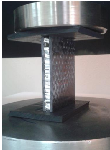
Figure 3.8. Edgewise compression specimen (Carbon fiber/epoxy composite/ Al honeycomb sandwich) under loading
