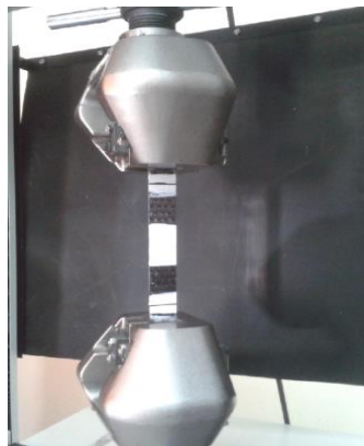
Figure 3.4. Tensile test specimen (composite face sheet) during the test
