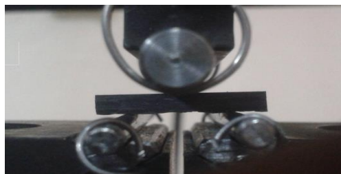
Figure 3.6. SBS test specimen and test configuration
