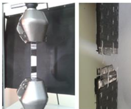
Figure 4.8. Tensile test specimen and set-up (left) and the failed test specimen (right)
