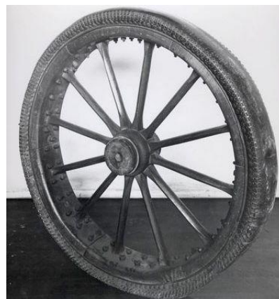
Figure 1.2. First pneumatic tire invented by Robert William Thomson (Source: http://blog.hemmings.com/index.php/2013/12/10/this-day-in-history-1845-robert-william-thomson-patents-the-pneumatic-tire/ )
