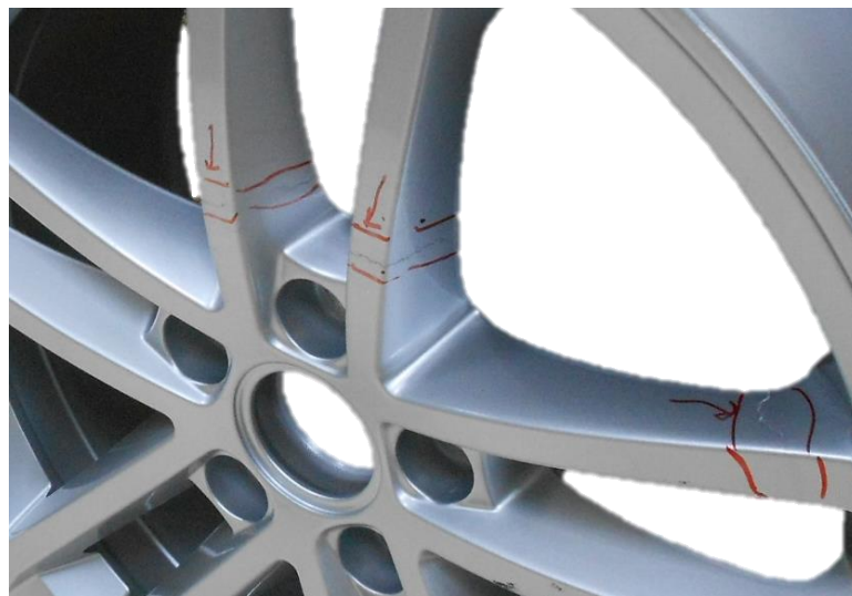
Figure.5.21 Experimental impact test result of the wheels under impact load 825 kg
