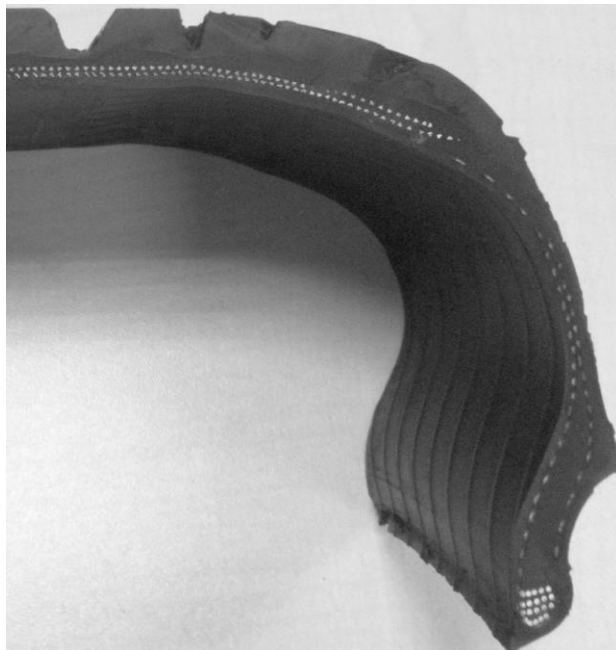
Figure 4.5. Half cross-section of the tire
