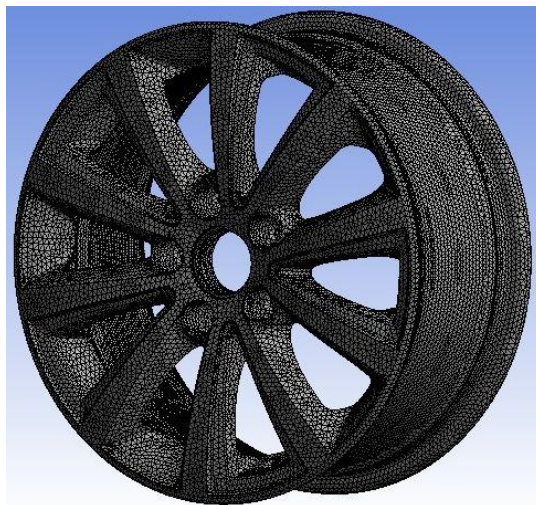
Figure 4.2. Finite element model of the wheel 1
