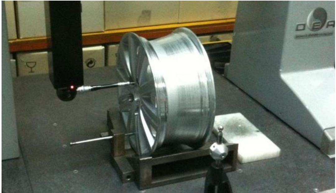
Figure 3.8. Measuring the plastic deformation by CMM
