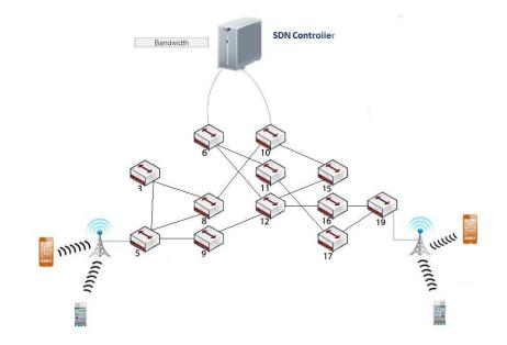
Figure 3.13. Demonstration of the second network with capacity per port of 200 Mbps after proposed routing for 8 flows with throughput requirements of 200 Mbps for the different source and destination nodes.
