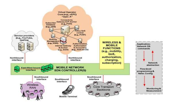
Figure 2.8. SDN-based mobile network interface architecture [Bernardos2014]
