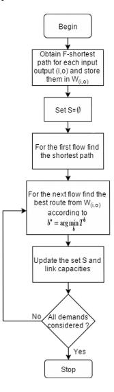
Figure 3.4. The flowchart of proposed routing algorithm
