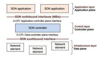
Figure 2.2. SDN components [ONF2014]
