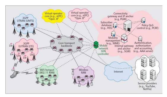
Figure 2.7. SDN-based mobile network architecture [Bernardos2014]
