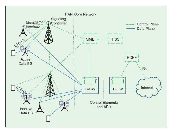
Figure 2.9. The integrated architecture [Zaidi2015]
