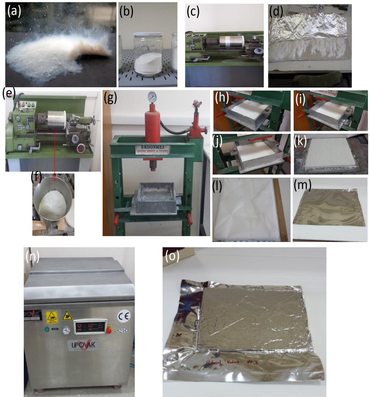
Figure 3.4. Pictures and processes for the production of vacuum insulating panels (a) Fumed silica as core material, (b) hollow nano calcite developed for this study, (c) winding the polyester binder for cut, (d) polyester cuts, (e) mixing of core and binder materials, (f) mixer container, (g) moulding machine with press, (h) filling the core material in the moulding, (i-j) compressed core material for VIP, (k) moulded core material ready for VIP making, (l) inner envelope or primary cover material, (m) commercial Alumina-PET, (n) vacuum packing system, (o) product of different types of VIPs.
