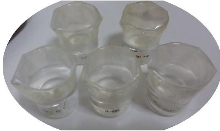
Figure 3.5. Water vapor transmission rate (WVTR) measurement system
