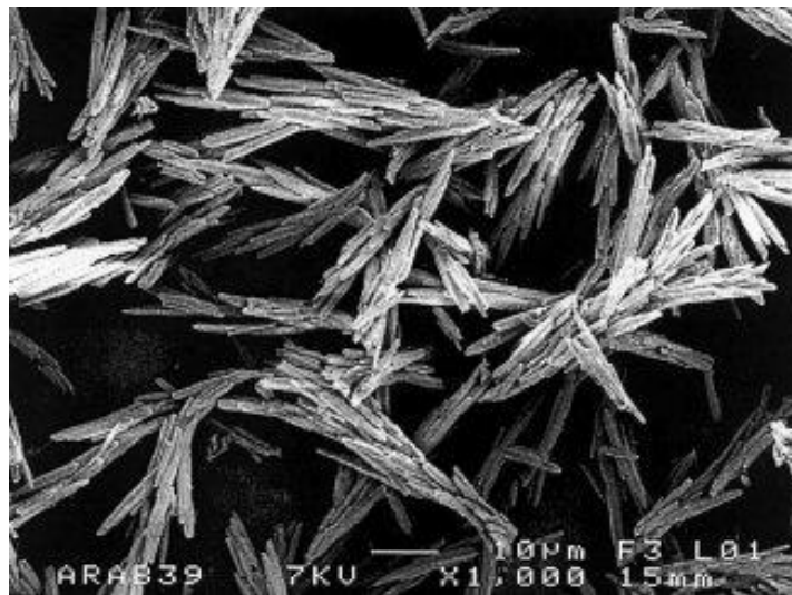
Figure 2.2. SEM image of aragonite crystals (Source: Lucas-Girot, Verdier et al. 2005)
