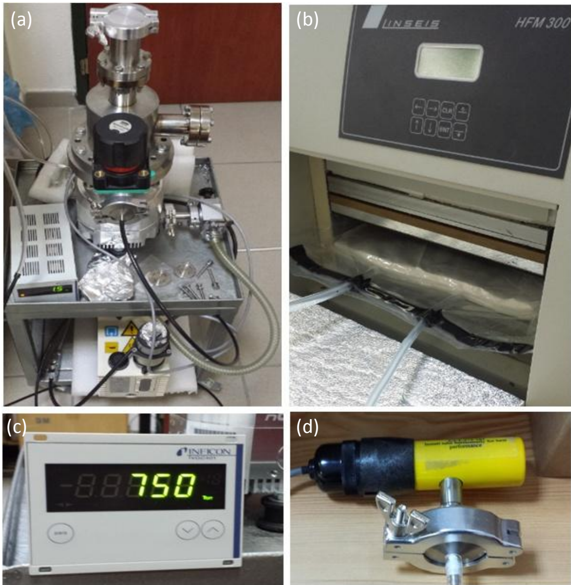
Figure 3.6. Thermal conductivity measurement equipment, (a) pump system, (b) thermal conductivity measurement device (Linseis HFM 300), (c) pressure indicator panel, (d) pressure gage.
