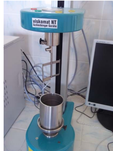
Figure 2: Rheometer and spindle geometry used in the experiments.
