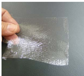
Figure 2: Biofilm made of PVA and recovered sericin-rich protein powder.
