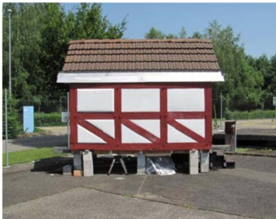
Figure 8: Prototype situated at EMPA Campus which is used for weathering tests.
