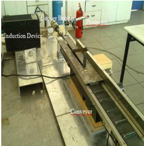
Figure 1: Induction Sintering Mechanism
