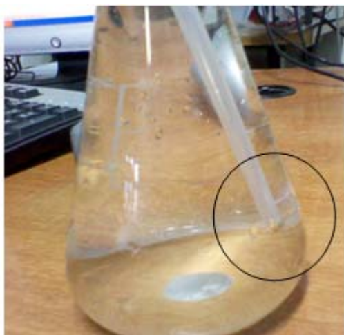
Figure 5: The control of the bubbles formed from the CO 2 permeation through the block samples.
