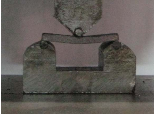
Figure 2: The TRS test setup.
