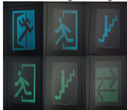
Figure 2: Images of produced photoluminescent tiles in dark
