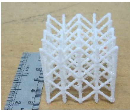
Figure 4: Cellular lattice structures fabricated by the FDM.
