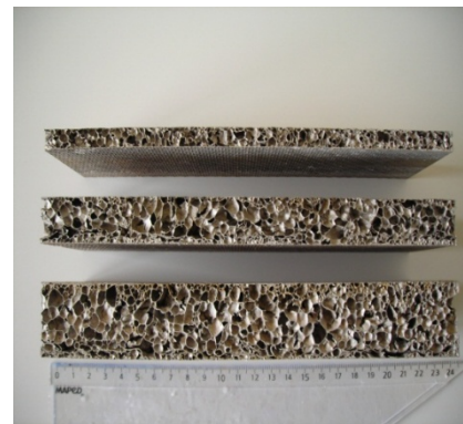
Figure 1: As-received ALULIGHT™ AFS Al foam panels with 8, 20 and 30 mm thickness.
