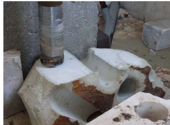
Figure 1: The sampling stage of zeolite blocks.
