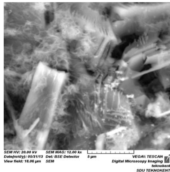
Figure 3: Chalk coccoliths make mechanically weak “mosaic” pore walls.
