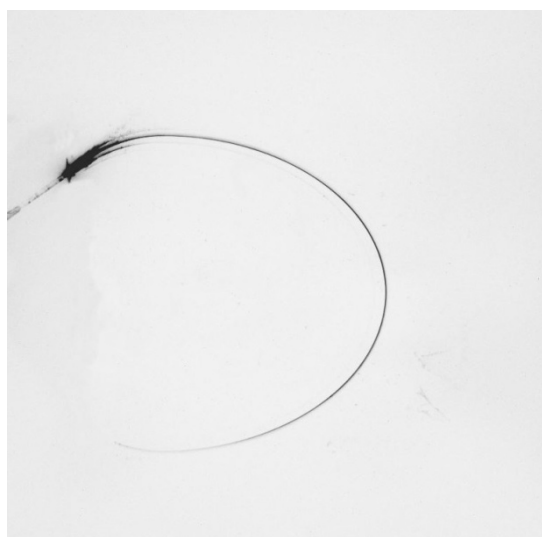
Figure 5: The photograph of 975 nm light propagation in the circular planar waveguide with embedded nano-phosphors.
