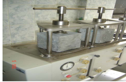
Figure 2: Pressurized water permeability test
