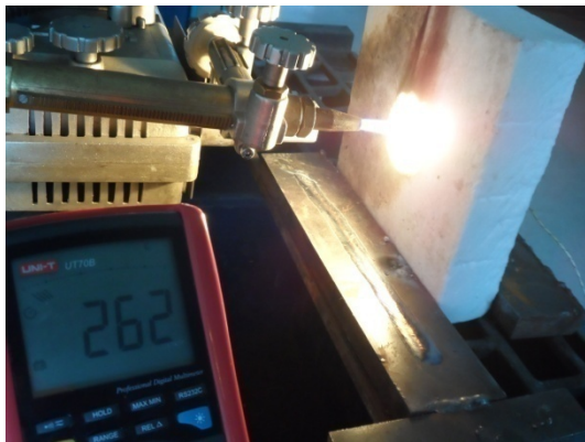
Figure 2: Ablation test set-up.
