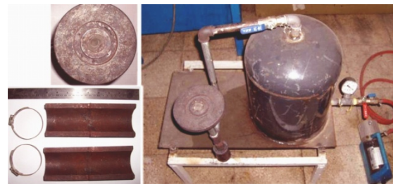
Figure 1: Vacuum casting system and casting mould.
