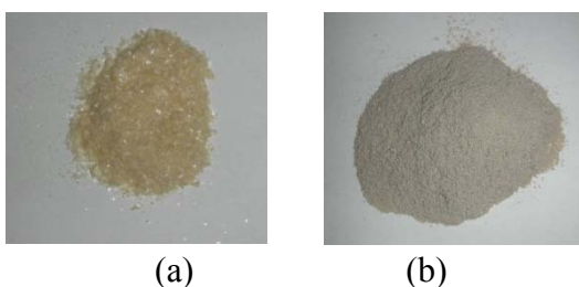
Figure 1: Powder sericin; (a) commercial (b) recovered from wastewater.
