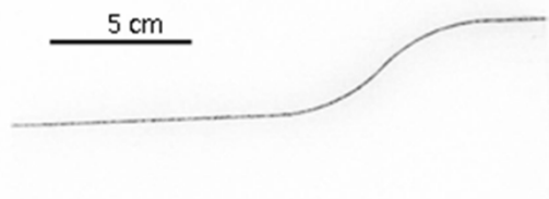
Figure 4: The photograph of 975 nm light in the s-shape planar waveguide with embedded nano-phosphors.
