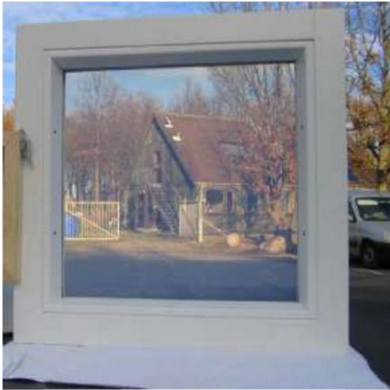
Figure 7: Aerogel window glazing produced by HILIT + project.
