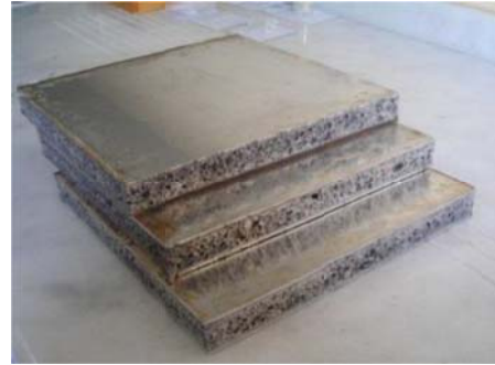
Figure 2: 30 mm thick Al/Al foam / GFPP sandwich panels fabricated.
