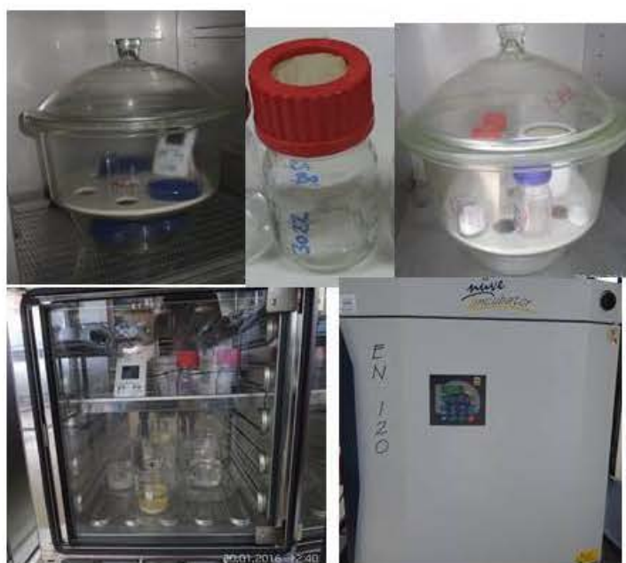
Figure 4.5 WVTR testing apparatus (cells, desiccator and oven)
