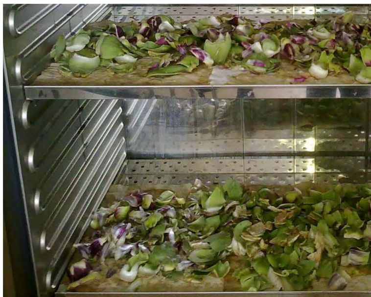
Figure 4.2 Drying artichoke leaves at 40°C for 24 h in fanned oven
