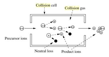
Figure 1.9. The principle of CID. (Source: (Eidhammer et al., 2008d)).
