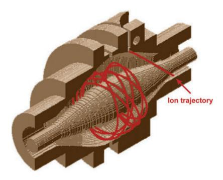
Figure 1.10. Ion trajectory shown by schematic diagram of the Orbitrap. (Source: (Hu et al., 2005)).
