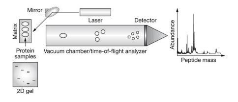
Figure 1.6. MALDI-TOF instrument setup. Here the analyte acquired from 2d gel is coupled with a matrix. Laser beams ionize the molecules which then enter a vacuum chamber and as soon as they hit the detector, according to their retention time, assigned a m/z value. (Source: (Din et al., 2007))
