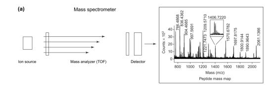
Figure 1.1. A mass spectrometer performing the first stage of mass spectrometry. This stage requires three devices: an ionization source, mass analyser and an ion detector. In this system the ions pass through the mass analyser from ion source to detector which takes a certain amount of time (time-of-flight) that will be used to calculate ions m/z value. (Source: (Yates, 2000))
