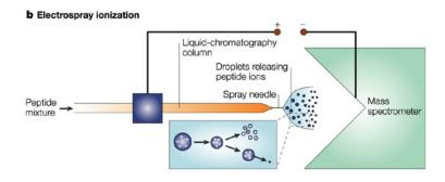
Figure 1.7. ESI workflow (Source: (Steen and Mann, 2004))
