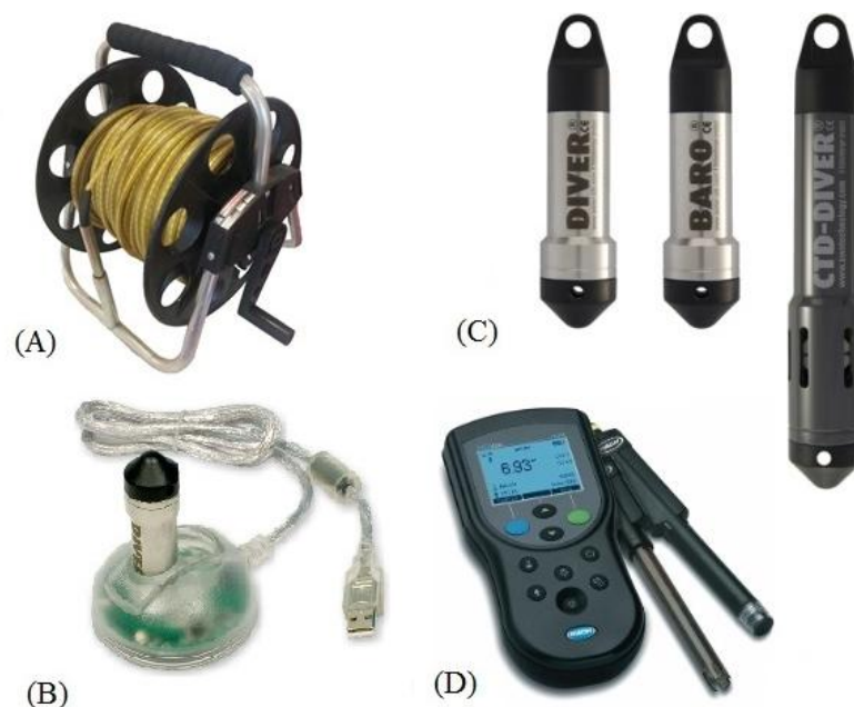
Figure 3.6. Examples of groundwater level measurement instruments. (A) Manual meter. (B) USB Reading Unit. (C) Different types of data loggers. (D) Multi Parameter Meter
