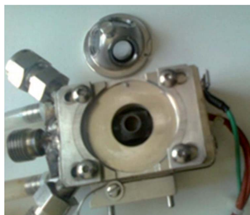
Fig. 3 Harricks in situ reaction cell with \text{CaF}_2 windows.
