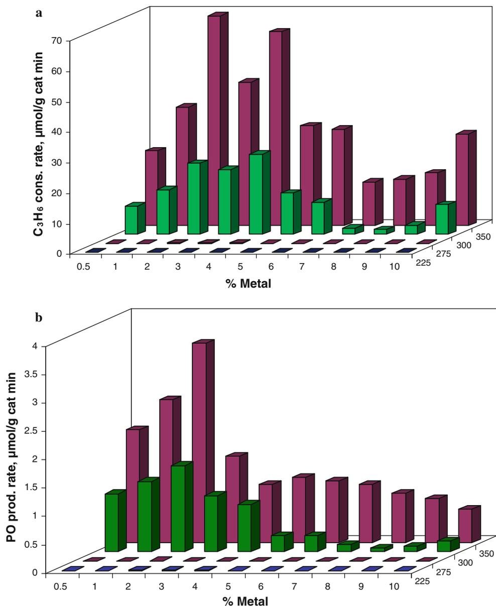
**Fig. 3** **a** Overall consumption and **b** PO production rate of un-promoted Cu/SiO<sub>2</sub> catalysts as a function of metal loading at different reaction temperatures
