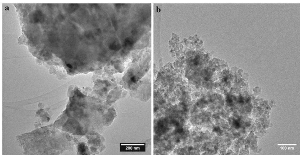
**Fig. 2** TEM image of **a** 1 % Cu-SiO<sub>2</sub> and **b** 3 % Cu-m-SiO<sub>2</sub> catalysts
