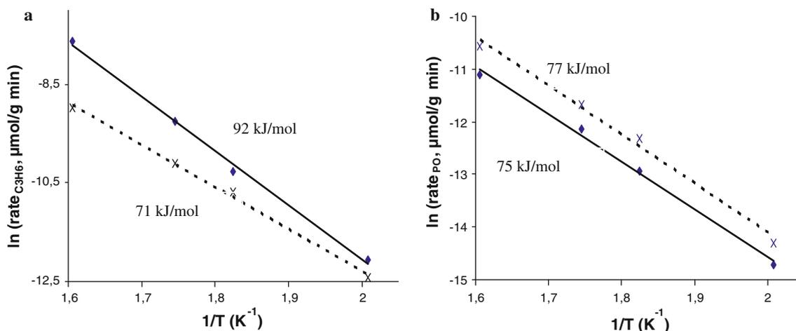
**Fig. 7** Arrhenius plots for the oxidation of propene (**a**) and PO production (**b**) over 3 % Cu/m-SiO<sub>2</sub> (straight line) and 3 % Cu-2.25 % K/m-SiO<sub>2</sub> (dashed line) catalysts
