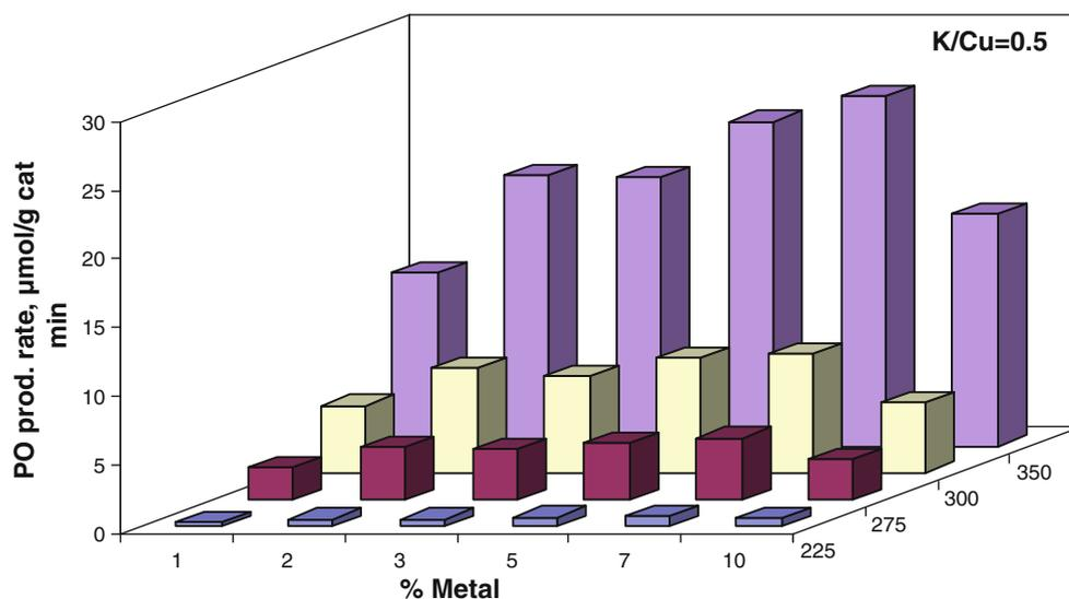
**Fig. 5** PO production rate for modified Cu catalysts at a K/Cu ratio of 0.5
