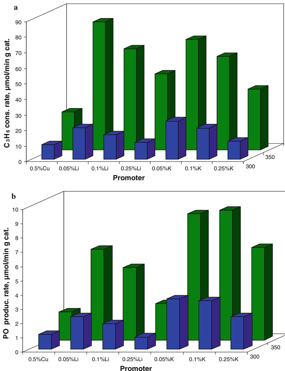
**Fig. 4** **a** Overall consumption and **b** PO production rate of K and Li-promoted 0.5 % Cu/SiO<sub>2</sub> catalysts at 300–350 °C
