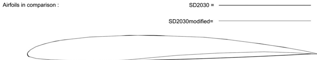
Fig. 12. Airfoil geometry comparison (SD2030 and modified).
