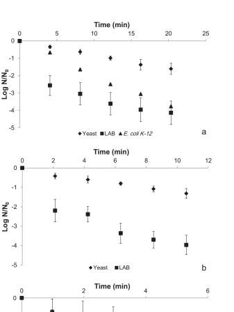
**FIG. 2.** UV INACTIVATION OF YEAST, LACTIC ACID BACTERIA (LAB) AND *ESCHERICHIA COLI* K-12 IN FRESHLY SQUEEZED TURBID GRAPE JUICE: (A) Q = 0.90 ML/S; (B) Q = 1.75 ML/S; AND (C) Q = 3.70 ML/S
