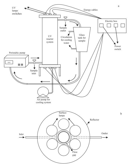
FIG. 1. (A) SCHEMATIC VIEW OF CONTINUOUS FLOW S-SHAPED UV SYSTEM WITH FLOW DIRECTION (B) LAMP CONFIGURATION (TOP-VIEW)
