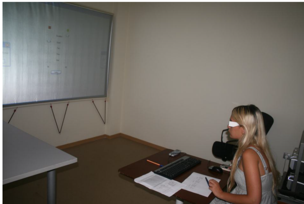
Figure 1. Stereo projection display laboratory: a special-purpose dark room consistent with the specifications given in ITU-R Rec. 500-11 [19].
