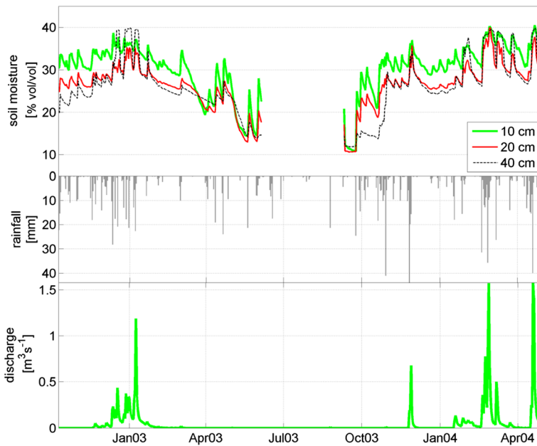
Fig. 2 Temporal variations of soil moisture at three different depths (10, 20 and 40 cm), daily rainfall and daily discharge in Colorso catchment for the period from October 2002 through to April 2004
