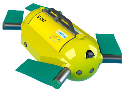
Fig. 5. The biomimetic AUV U-CAT
