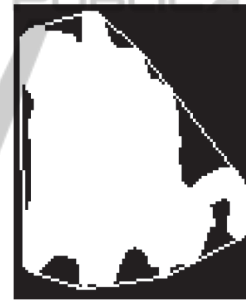
Figure 4: An example of an extracted silhouette and its convex hull. It is extracted from a motorcycle example using a single frame and its convexity is computed as 0.73 which is lower than the threshold \rho = 0.75 .
