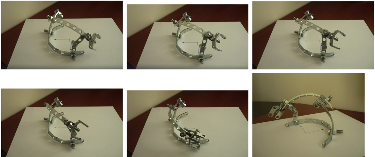
Fig. 7. The constructed spherical four-bar mechanism at different poses.
