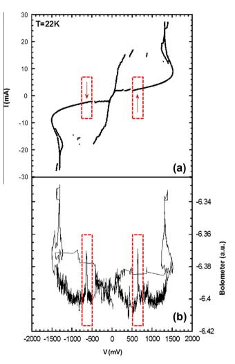
Fig. 3. I-V (a) and bolometer (b) measurements of mesa at 22 K.
