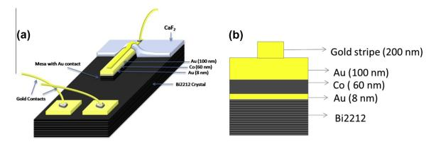
Fig. 1. Measurement configuration of the mesa structure (a) and the cross section of multilayer electrodes (b).
