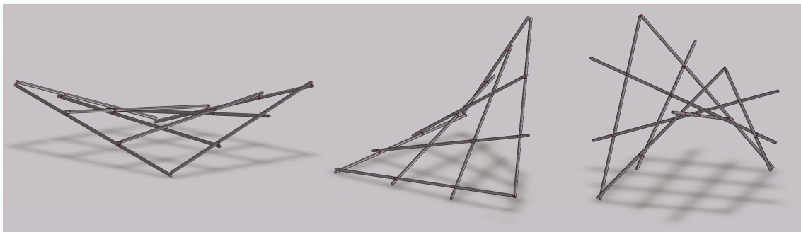
Figure 9. Three different deployed configurations of 2DoF 3x3-unit HP structure
