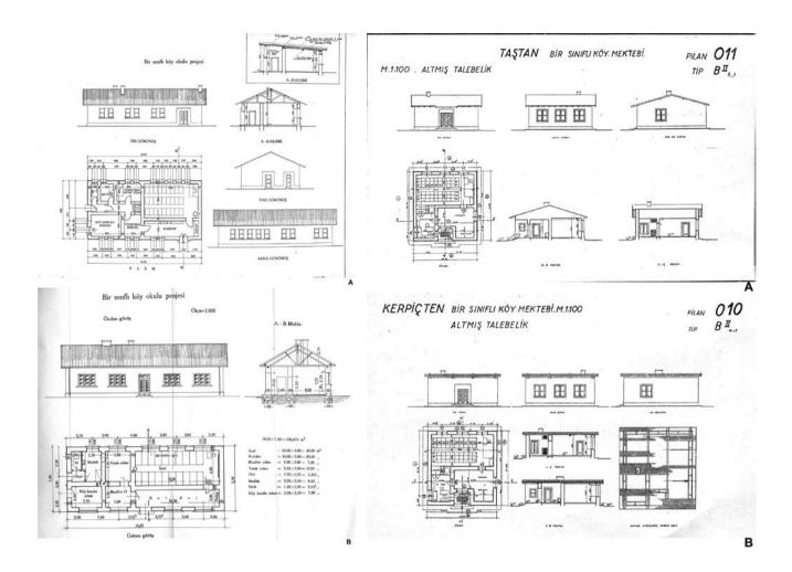
Figure 6. Two similar prototype designs of the Ministry of Education for village educators. Both designs were to be constructed in different regions with different construction material alternatives such as stone, brick, mud-brick and timber, compatible with the climatic conditions and available material alternatives of that region (Köy Okulu Binası, 1937).
