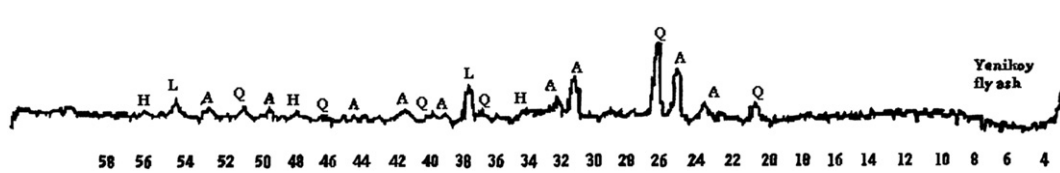
Fig. 2. XRD analysis results of the ash samples (Q = quartz ( \text{SiO}_2 ), A = anhydrite ( \text{CaSO}_4 ), L = lime ( \text{CaO} ), H = hematite ( \text{Fe}_2\text{O}_3 )).
