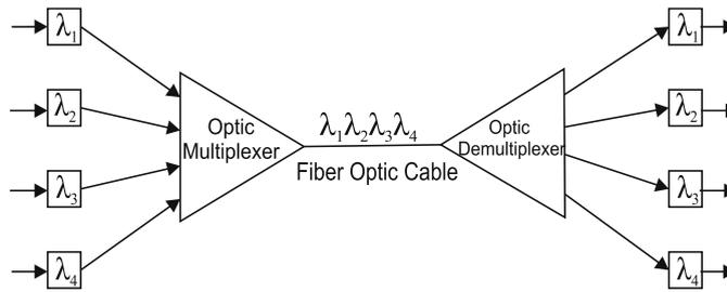
Fig. 1. A simple WDM system with 4 wavelengths.
