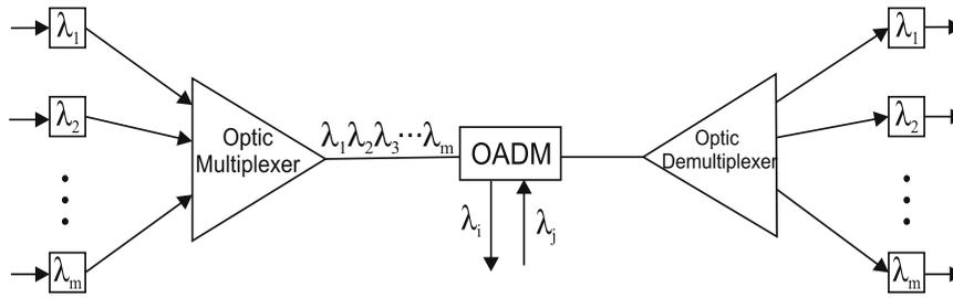
Fig. 2. OADM in a DWDM system.
