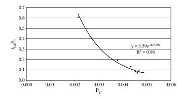
**Fig. 7.** Variation of lag time,  $t_{\text{lag}}/t_r$ , with unsteadiness parameter,  $P_{gt}$
