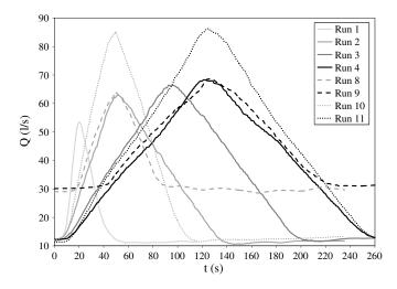
**Fig. 1.** Variation of discharge with time for different hydrographs (Runs # 1–4 and 8–11)
