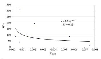
**Fig. 4.** Variation of modified unsteadiness parameter, *P*, with nondimensionalized total bed load,  $W_i^*$
