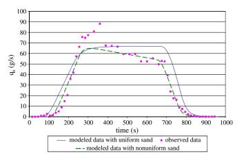
**Fig. 10.** Comparison of numerically modeled sediment yield with uniform and nonuniform bed material with observed sediment yield at downstream of flume after trapezoidal hydrograph
