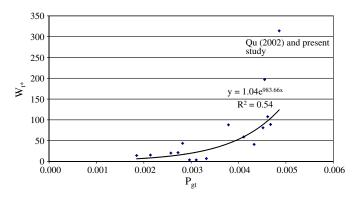
**Fig. 6.** Variation of nondimensionalized total bed load,  $W_t^*$ , with proposed unsteadiness parameter,  $P_{gt}$ , for present study and Qu (2002)
