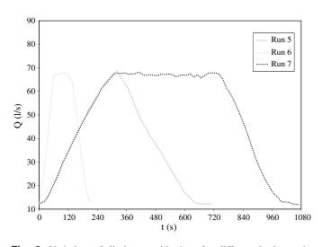
**Fig. 2.** Variation of discharge with time for different hydrographs (Runs # 5, 6, and 7)
