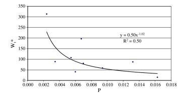
**Fig. 3.** Variation of unsteadiness parameter, P, with nondimensionalized total bed load,  $W_i^*$
