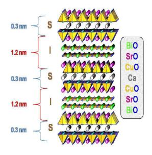
Fig. 1 Generic view of Bi<sub>2</sub>Sr<sub>2</sub>CaCu<sub>2</sub>O<sub>8+δ</sub> (Bi2212) crystal.
